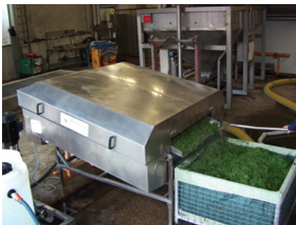
A Baleen filter installed for Algae recovery
